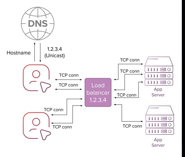
Layer 7 load balancing – "reverse proxy"
