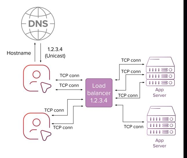
Layer 7 load balancing – "reverse proxy"
